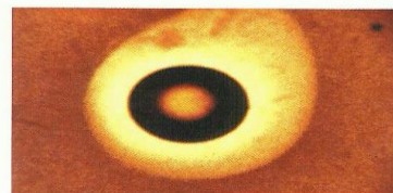
Fig. 9.8 Asymmetric exclusion zone around a gel bead, resulting from incident light coming from top right.
